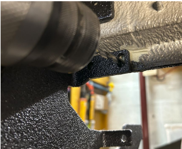
4.1 Drill through the vehicle flange using a 1/4" metal drill bit at the center of the slotted hole located at the bottom of the brackets.
