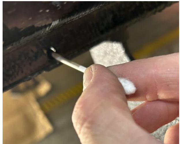
4.2 Apply metal paint inside the hole.
