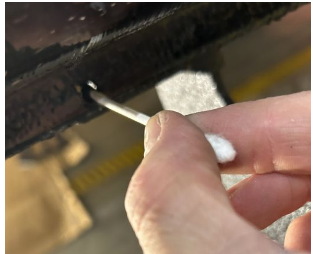
5.2 Apply metal paint to the hole
