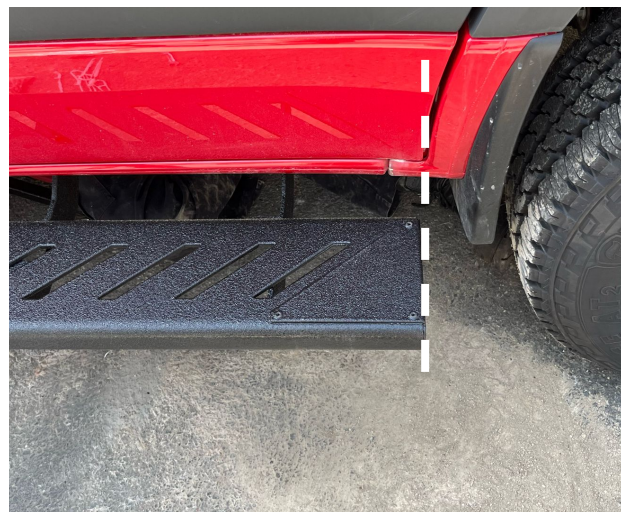
8.2 Adjust the front-to-rear position of the side steps. Align them with the front edge of the front passenger door.
