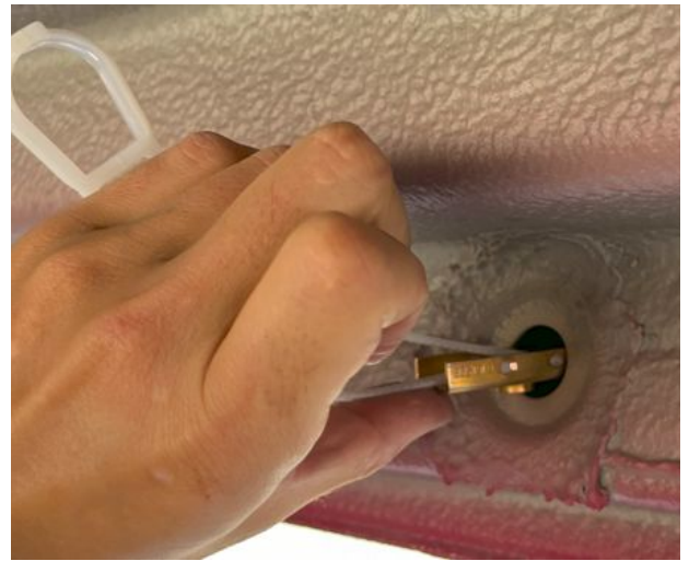
3.2 Gently pull the serrated straps until the washer is seated against the vehicle
