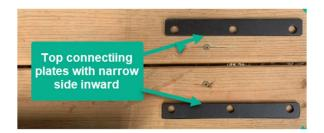
3.1 Manually align the front and rear side plates as straight as possible.
