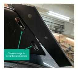
5.2.6. Tighten the 4 bolts/nuts assemblies to a torque of **16 N·m** using a torque wrench.
