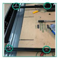
1.2. Position the spring nuts at the same distance as the assembly holes of your solar panel to be installed.
