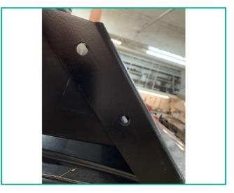
5.2.2.Insert the 3/8"-16 x 1" bolts through the wind fairing and than the side plate.
