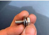
1.6. Insert the assembly through the solar panel and manually screw into a spring nut.
