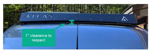
To adjust this clearance, raise the wind fairing higher than the side plates using the oblong holes allowing this adjustment.
