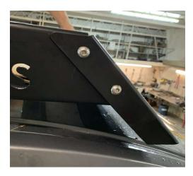
5.2.3.Insert a 3/8" flat washer and a nylon lock nut 3/8" on the bolts.
