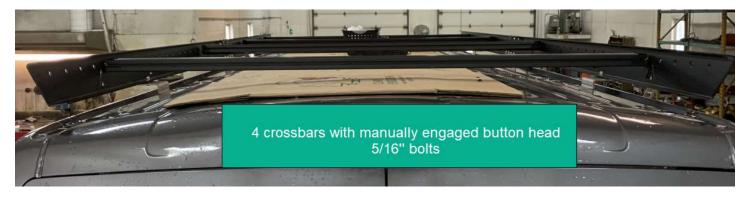
4.7 Tighten the 8 crossbar bolts to a torque of **12 N·m** using a torque wrench.
