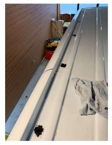
1.5 Liberally apply a bead (about 1/2" bead diameter) of SikaFlex221 around the entire circumference of the bores. The joint of Sika221 must be as uniform as possible and seal the circumference of the hole.
