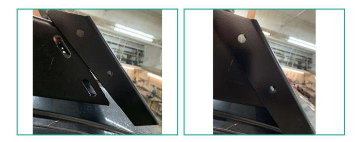
5.2.2.Insert the  $3/8''-16 \times 1''$  bolts through the wind fairing and than the side plate.
