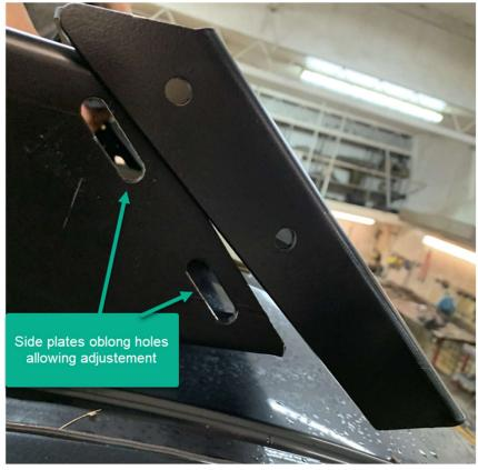
5.2.6.Tighten the 4 bolts/nuts assemblies to a torque of **16 N**•**m** using a torque wrench.
