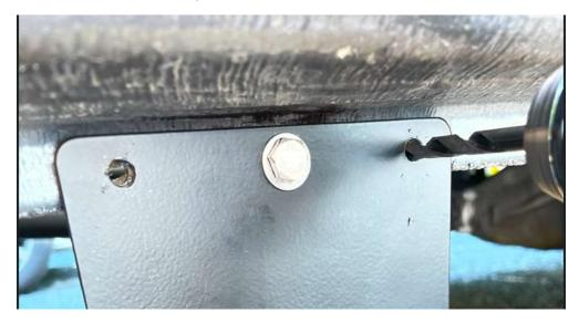
5.3 Drill the 3 assembly holes using a 9/32" metal bit.
