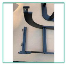
1.2. Remove central rung of the ladder by unscrewing the 2  $\frac{1}{2}$  -20 x  $\frac{3}{4}$  bolts.
