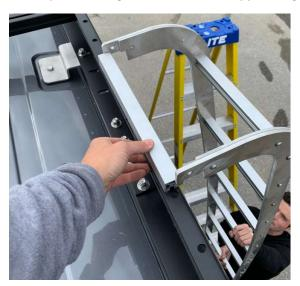
3.2 Put a drop of LOCTITE 242 or LOXEAL 54-03 adhesive on the end of the two 1/4"-20 x 3/4" bolts previously removed and manually insert them through the ladder's stiles. Do not tighten completely right away.
