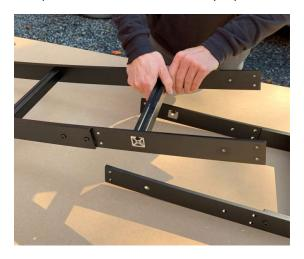
1.4. Place the to ladder sections end to end aligning all holes as accurately as possible.
