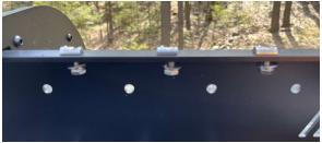
2.3. Carefully slide the T-nuts into the upper rung slot until the nuts are centered in the rung.
