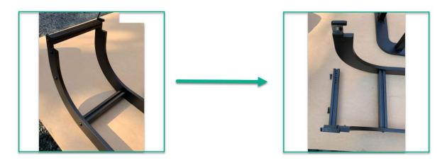
1.2. Remove central rung of the ladder by unscrewing the 2 % 20 x % bolts.
