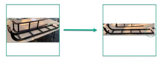
1.3. Insert the central rung into the square holes intended for this purpose.
