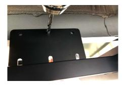
5.5 Insert a flat washer on a 1/4"-20 x 1" hex head bolt. Insert the assembly through the metal lip and the connecting plate. The assembly must be inserted from the outside of the metal lip (under the plastic molding) to the inside of the vehicle.
