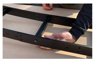
1.6. Put a drop of threadlocker on the ten 1/4" -20 x 1/2" bolts. Manually insert all bolts by aligning the 2 ladder sections together.
