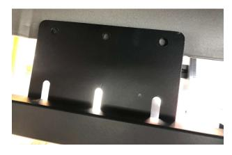
5.4 Drill the 3 assembly holes using a 9/32" metal bit.
