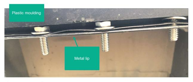
5.6 Insert a flat washer and a  $\frac{1}{4}$ " nylock on the bolt.
